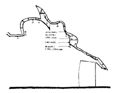
Figure 1. Section Diagram of EMP's structural and cladding system
